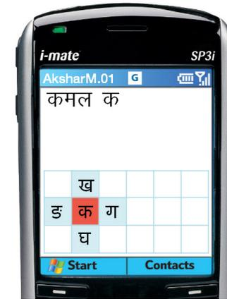
**figure 5:** Visual feedback available on the mobile device when number 2 on the keypad is pressed.
