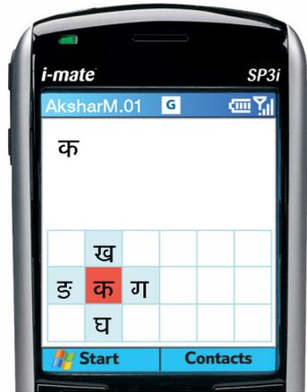
**figure 8:** Visual feedback available on the mobile device when number 2 on the keypad is pressed.
