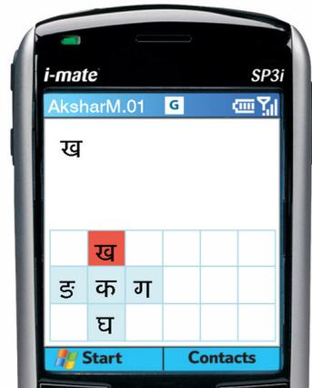
**figure 9:** Visual feedback available on the mobile device when number 2 on the keypad is pressed, followed by the up arrow key.
