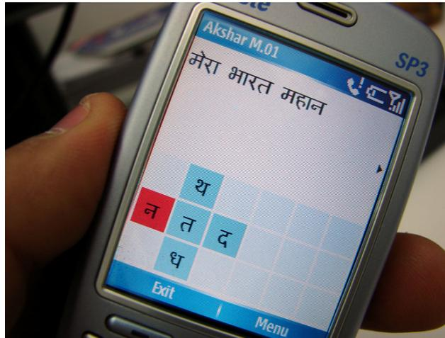
**figure 14:** Working prototype of the AKSHAR.
